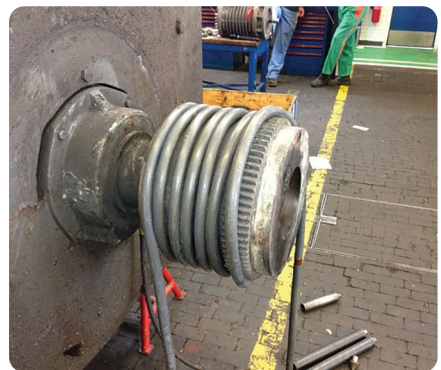
Heating a coupling for dismantling
