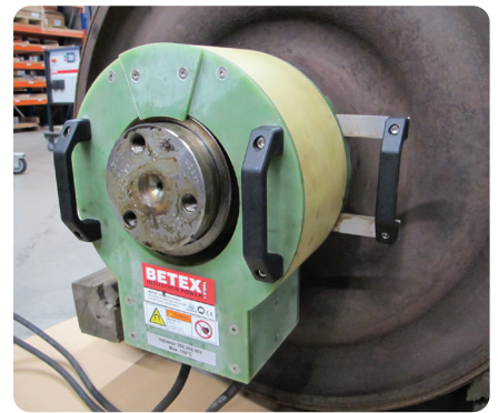
Heating bearing rings for dismantling
