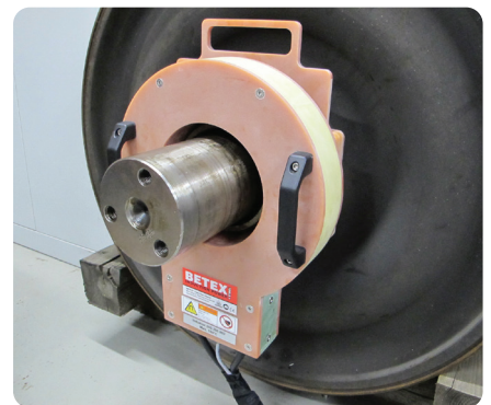
Heating labyrinth rings for dismantling
